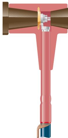
T-adapter for perpendicular connection of the termination to SF<sub>6</sub>-insulated switchgear
